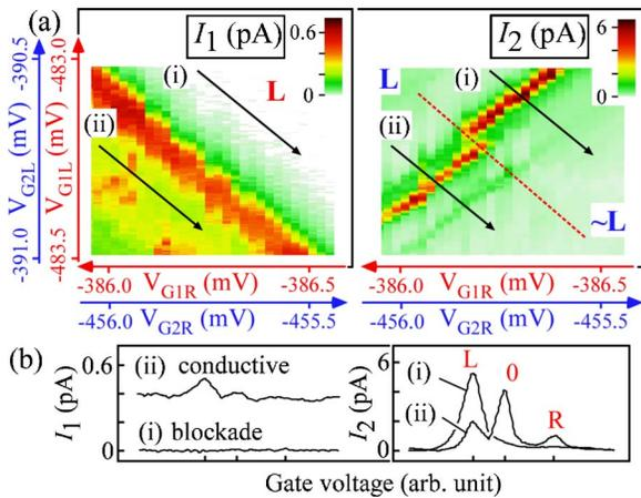
FIG. 3. (Color online) (a)  $I_1$  and  $I_2$  simultaneously obtained with the two-dimensional sweep of  $V_{G2L}$  and  $V_{G1L}$  for the vertical (y) axis and  $V_{G2R}$  and  $V_{G1R}$  for the horizontal (x) axis. (b)  $I_1$  and  $I_2$  traces along lines (i) and (ii) in (a). The gate voltages are different from that in Fig. 2, since the data set was measured after a thermal cycle up to room temperature.
